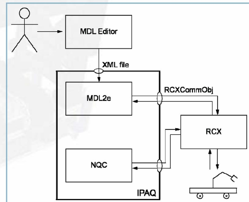
Figure 2: Behaviour based control of the LEGO robot
