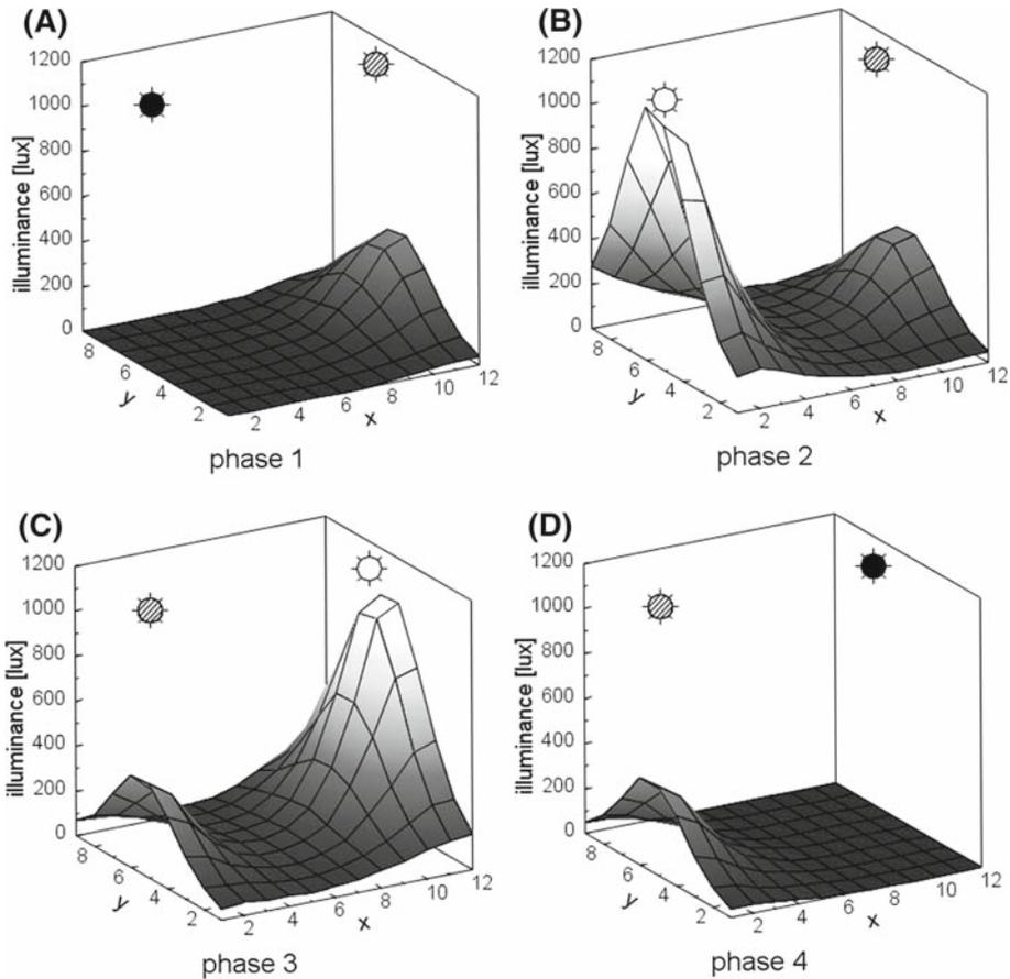
**Fig. 7** Spatial distribution of illuminance in the arena during the four distinct phases of our experiments in the dynamic environment. The small sun-like symbols in the upper sections of the graphs represent the lights’ intensities at the respective light. A striped sun indicates that the light was dimmed; a white sun indicates that the light was bright and the black sun indicates that the light was switched off
