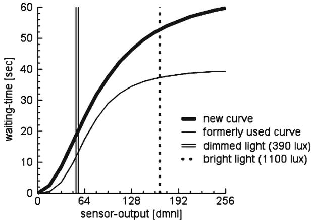
**Fig. 8** Dependency of the duration of the state “wait” on the local illuminance measured by the robot. The bold curve indicates the function used in the experiments described in this article, the thin curve depicts the function used in [26]. The dotted vertical line indicates the median illuminance measured by the robots directly below a bright light; the vertical parallel line indicates the medium illuminance measured by the robots directly below a dimmed light
