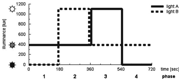
**Fig. 6** Timing of our experiments focussing on the behaviour of the robotic swarm in a dynamic environment. Every 180 s the lights’ intensities were modified, thus changing the environmental conditions for the robotic swarm
